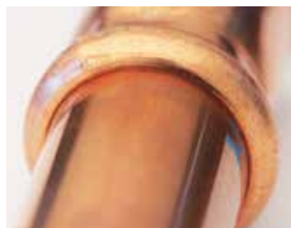
Pressed fitting - no gap between fitting and tube.
