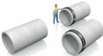
Position plain ended pipes.
