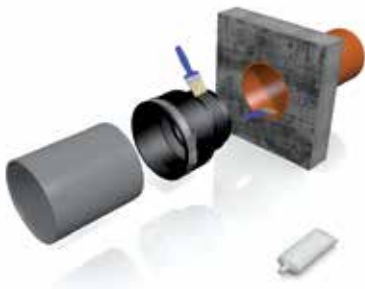
Position pipe ends.
