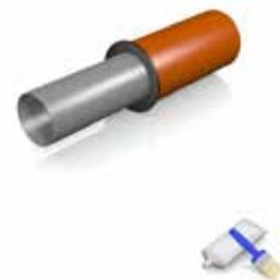
Insert smaller pipe into Single Pipe Connector.
